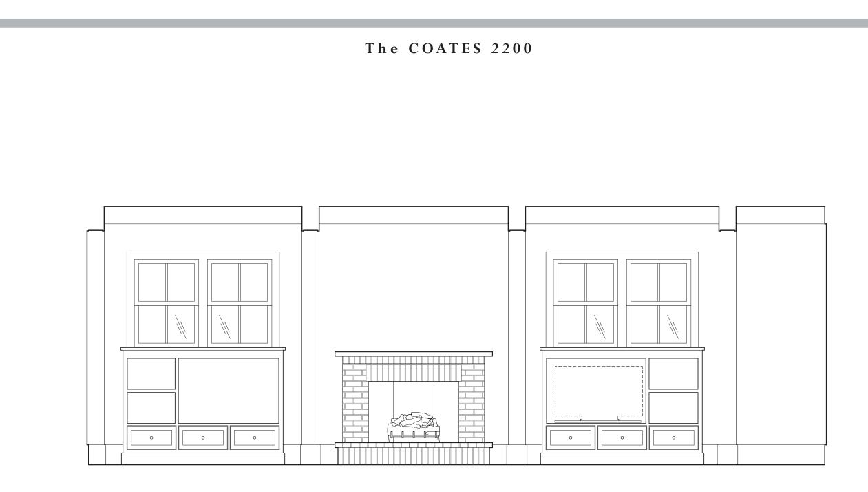
Built-In Cabinetry - Elevation
